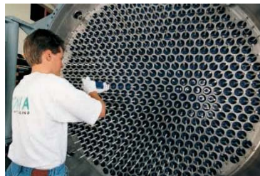
Ozone generation for water cleaning
